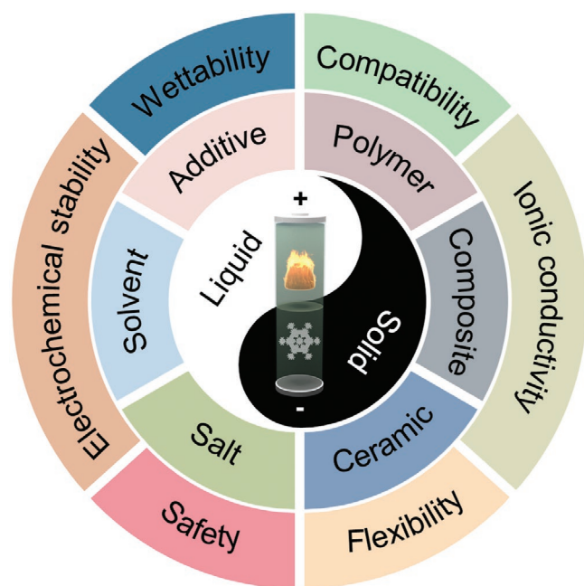
Figure 1. Compositions, properties, and requirements of the electrolytes used for batteries capable of operating over wide temperature windows.
